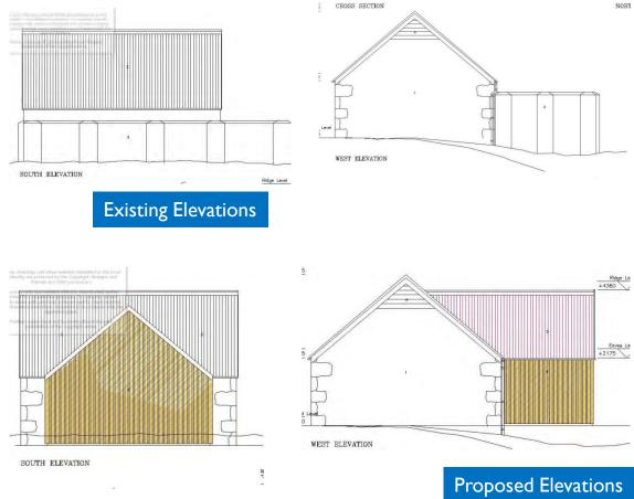
•Full planning permission is sought for a pitched roof extension to an existing agricultural outbuilding to house equipment including ground source heat pump.
